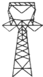
500 kV Lattice Average height 135' Average span 1150'
