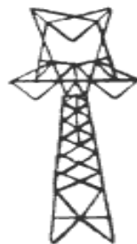
500 kV Lattice Average height 125' Average span 1150'
